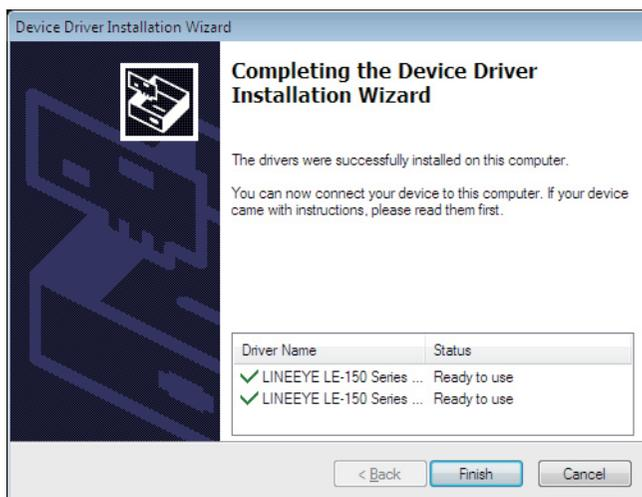
8. Connect LE-150P device to the PC. If the PC can recognize the device, the message like below will be displayed. When you connect to the different USB port, same thing will happen again.
