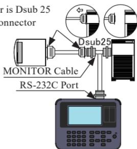
If the connector of either target device is Dsub 25 pin, use attached Dsub 25 pin monitor cable (LE-25M1) to connect to the analyzer.
