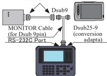
If the connectors of both target devices are Dsub 9 pin, use attached Dsub 9 pin monitor cable (LE-009M2) and Dsub 25-9 conversion adapter to connect to the analyzer.
