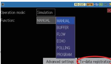
Touch "Tx-data registration" to register the data to be used in the simulation function.
