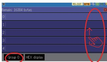
Input the data to be transmitted in HEX by [0] to [F].
