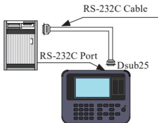
DTE device -----Straight cable -----Analyzer (DCE setting)
