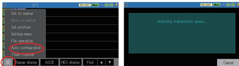
When the communication conditions are determined, the details will be displayed. A few seconds after that, the current communication condition settings are automatically changed to the determined communication conditions and it starts the measurement.
