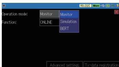
"Depending on the function, touch "Advanced settings" or press [ENTER] to configure the operational condition.
