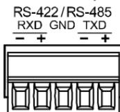
\*This is the removable terminal. Remove it from analyzer first, connect cables and return it to the analyzer.
