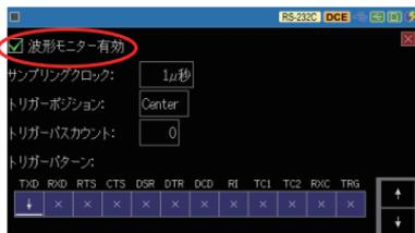
Set the sampling clock to approximately 5 times the communication speed as a guide.
