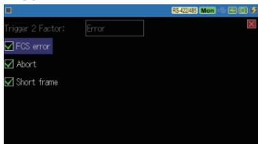
FCS (Frame Check Sequence) error, Abort (continuous 1 more than 7bits) and Short frame (less than 3 characters) are the trigger factor. Selected errors will be detected.
