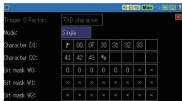
Set the character string. Up to 8 characters can be set for each of D1 and D2, and \* (don't care) and bit mask (don't care by bit unit and 3 types of W0 to W2) can be set.
