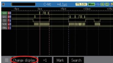
To change to logic analyzer display, touch “Change Display”. (Set and measure the wave monitor in advance.)
