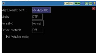
From the top menu screen, touch “Interface” or press [1] to configure at the interface port setting screen.
