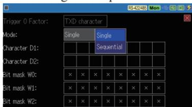
Single action means when Character D1 or D2 happens, the trigger will work.
