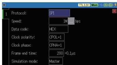
From the top menu screen, touch “Configuration” or press [0] to configure at the configuration display.
