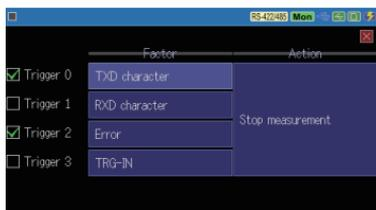
It can automatically stop the measurement when a specific trigger factor is detected during measurement operation. From the top menu screen, touch “Trigger” or press [2] to display the trigger selection screen.
