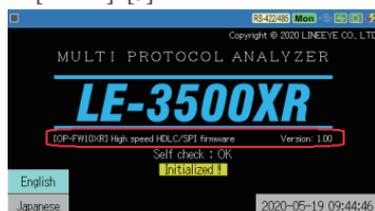
Save your important data in the SD cards before changing the firmware mode. It will initialize the analyzer and erase all data when the analyzer changes the measuring mode.
