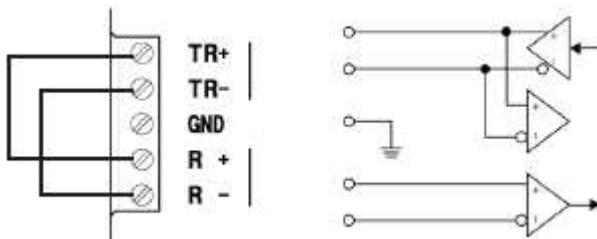
In case you do the test when SW-A No.4 is on, you need to make DTR signal active by the communications software before sending data.
