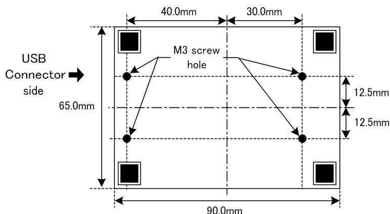
Notice: Use the screws that can be inserted less than 6mm from the surface line.
