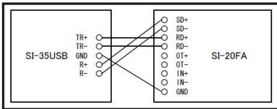
An example of N:N connection between RS-485 devices (between SI-35USBs)
