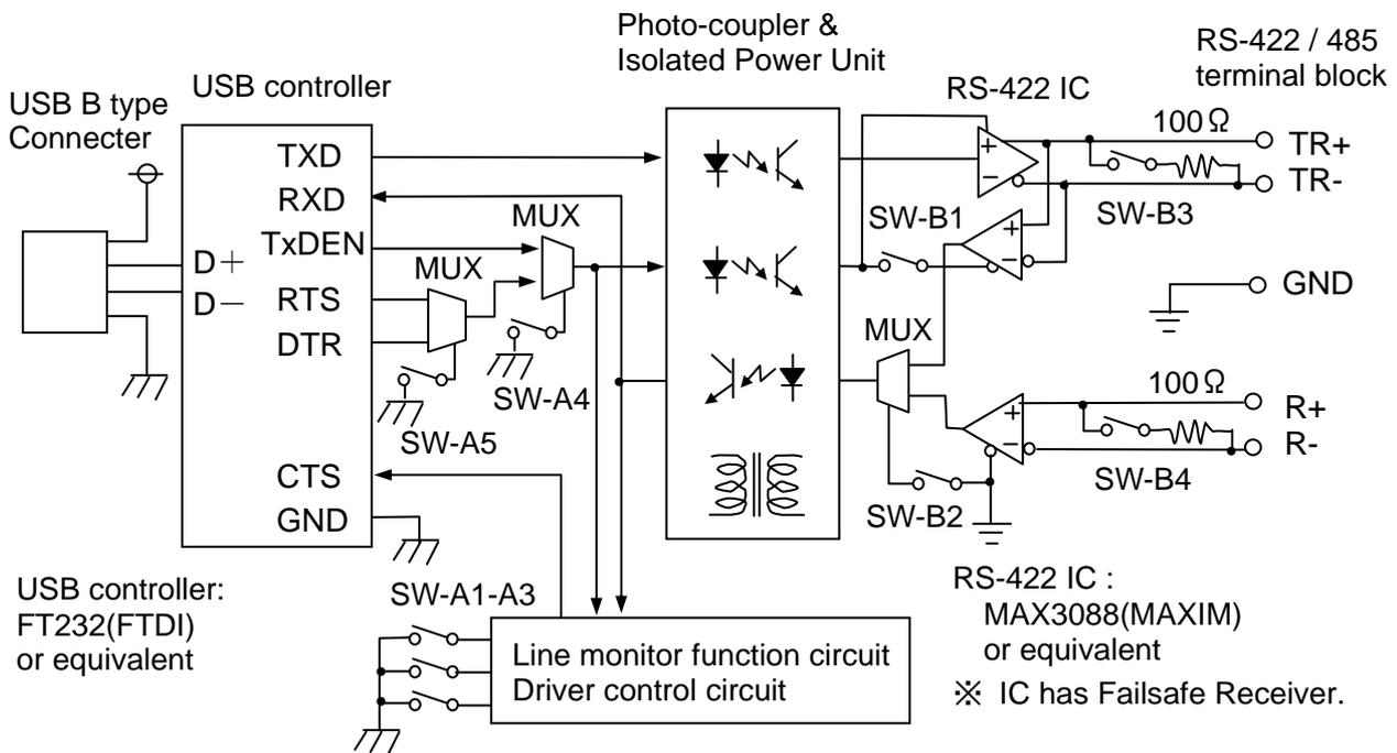
RS-485 communications of two-wire half duplex is required to send data after confirming that any devices have not sent data into the RS-485 line.
