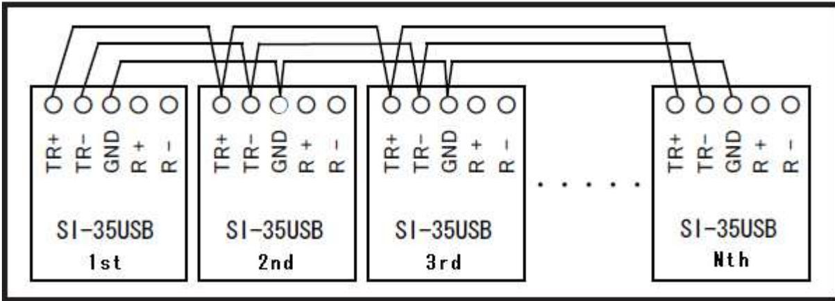
Maximum of 128 devices can be connected if constituted only by SI-35USB. (tested by LINEEYE)
